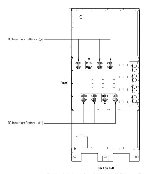
Figure 4-25. ISBM Section Power Terminal Detail BB – Common Battery
